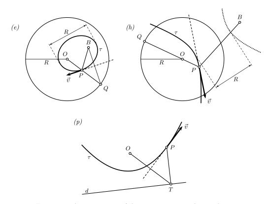
FIGURE 1. The construction of the trajectory  $\tau$  according to the sign of the energy: (e) if E < 0, the trajectory  $\tau$  is an ellipse, (h) if E > 0, the trajectory  $\tau$  is one branch of a hyperbola, (p) if E = 0, the trajectory  $\tau$  is a parabola.
