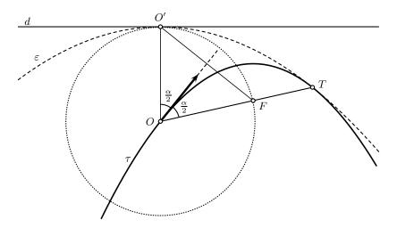
FIGURE 4. The envelope  $\varepsilon$  of all possible trajectories where the direction of  $\vec{v}_0$  varies but the magnitude  $v_0$  remains constant.
