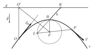
FIGURE 3. Parabolic trajectories in a homogeneous force field (indicated by the aceleration  $\vec{g}$ ).
