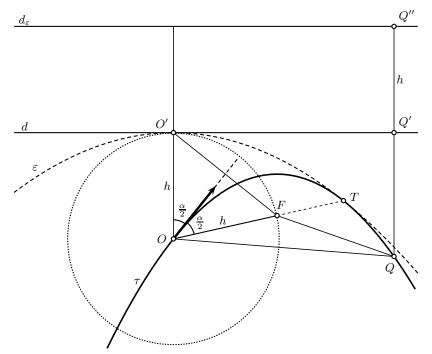
FIGURE 9. The envelope  $\varepsilon$  of all possible trajectories where the direction of  $\vec{v}_0$  varies but the magnitude  $v_0$  remains constant.
